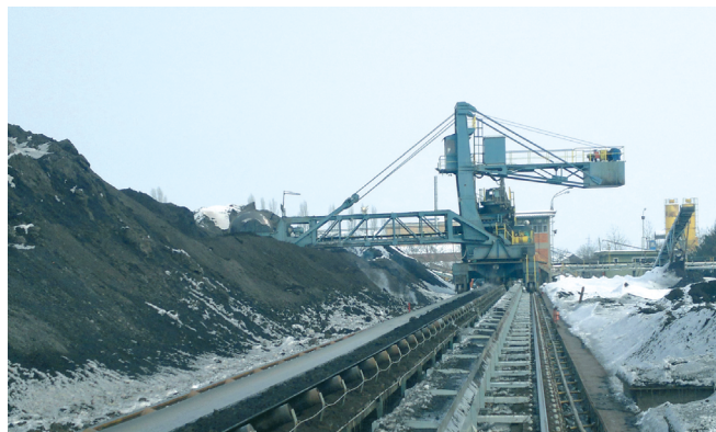
590.5 ft. (180 m) travel, 20.2 lbs/ft (30 kg/m) fill weight. Two igus® E4 Rol E-Chains®
